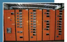
Being modular means the Moducell v2.2 system can be modified on site with the minimum interruption to power thus reducing operational and economic disadvantages. The switchboard is available in either 415/690/1000V configuration with bus bars and incomers rated up to 5000A 80kA fault level. The system is extremely flexible with the main bus located top/bottom/centre providing multi bus configurations and simplicity in design.
